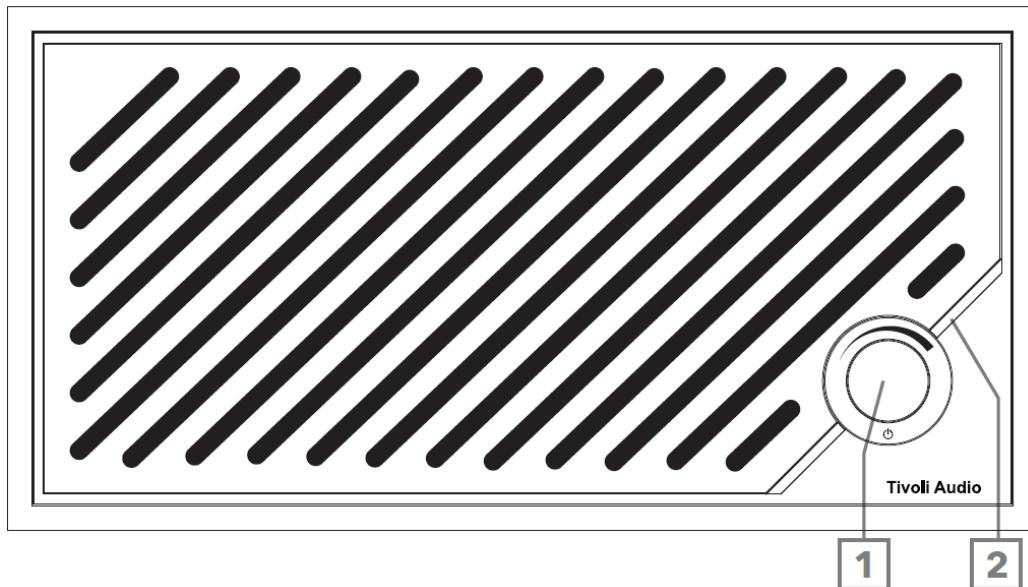
1. **POWER/SOURCE/VOLUME KNOB:** Short press to turn on, press and hold to turn off. Short press to cycle between Wi-Fi, Bluetooth and Aux In sources. Rotate right to increase volume, rotate left to decrease volume.
