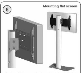
a bracket with three coupling boxes has to be mounted at the back of the flat screen (see specific mounting instructions flat screen brackets)
