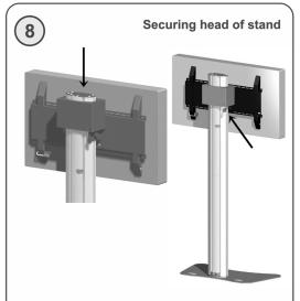
Slide the securing profile over the head of the stand (when cables come out of the top of the column the cables must be put firstly through the securing profile). The head of the stand and the securing profile can be locked with an optional anti-theft lock.
