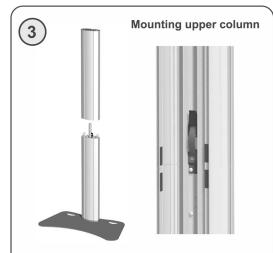
Place the upper column of the stand (cable duct closed) carefully on the bottom column. Use the latch to secure upper column of the stand to the bottom column.
